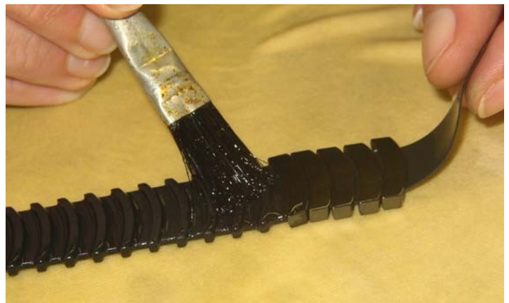
Paint the inlay with silicone oil and pull the links to their end position
